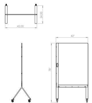
Dry Erase Board: Two sided durable dry erase surface with virtually no ghosting properties, tough 2mm PVC edge banding. Base & Frame: Powder Coated Steel for long lasting quality and protection against bumps and dents. Casters: Four swivel casters with breaks
